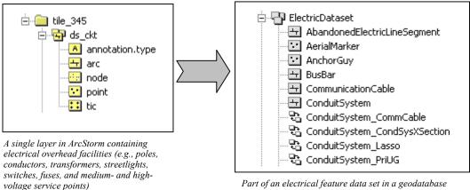
Part of an electrical feature data set in a geodatabase containing all electrical features in a seamless network (overhead and underground)
