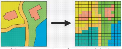
One of the most common types of raster data is land cover derived from satellite imagery. Land-cover data is produced by assigning each pixel in a Landsat thematic mapper image to one of 16 land-cover classes using a procedure known as unsupervised classification.
