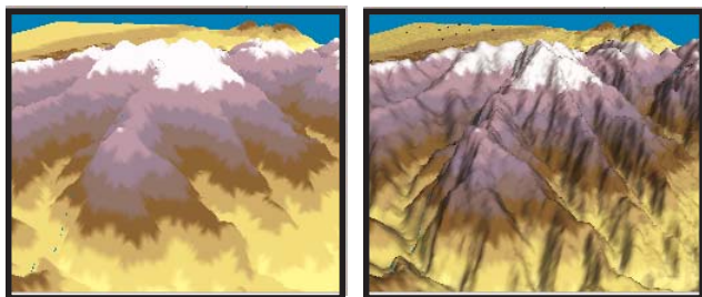
3D perspective view of terrain without and with hillshading
