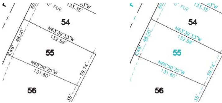
Raster image prior to selection (left); cell selection based on pixel area (right)
