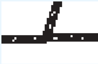
Raster lines containing holes
