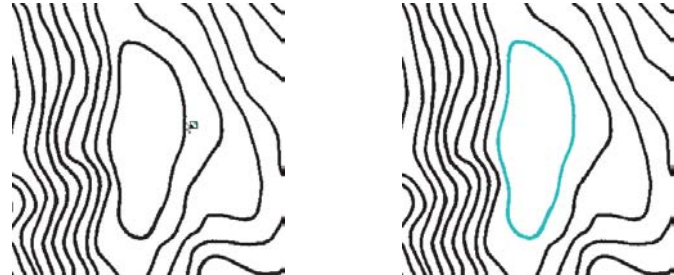
Raster display of contour lines (left); selected series of connected cells (right)
