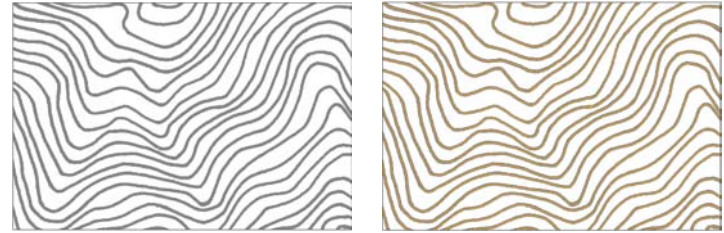
Raster display of contour lines; centerline vectorization of contour lines
