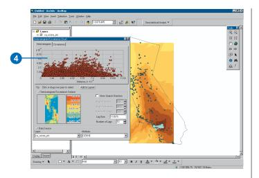
The pairs of sample locations that are selected in the semivariogram are highlighted on the map, and lines link the locations, indicating the pairing.
