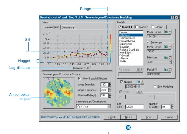
between pairs of points. Points separated by a lag distance greater than the range are spatially uncorrelated. The nugget represents measurement error and/or microscale variation (variation at spatial scales too fine to detect). It is possible to estimate the measurement error if you have multiple observations per location, or you can decompose the nugget into measurement error and microscale variation by checking the Nugget Error Modeling check box.
