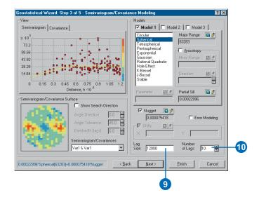
By removing the trend, the semivariogram will model the spatial autocorrelation among data points without having to consider the trend in the data. The trend will be automatically added back to the calculations before the final surface is produced.
