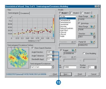
15. Type the following parameters for the Search direction to make the directional pointer coincide with the major axis of the anisotropical ellipse:
