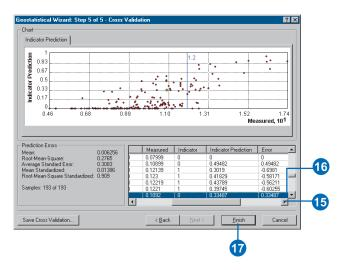
The measured and indicator columns display the actual and transformed values for each sample location. The indicator prediction values can be interpreted as the probability of exeeding the threshold. The indicator prediction values are calculated using the semivariogram modeled from the binary (0,1) data, created as indicator transformations of your original data. Cross-validation sequentially omits a point and then calculates indicator prediction values for each.
