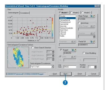
The Semivariogram/Covariance Modeling dialog box allows you to examine spatial relationships between measured points. You assume things that are close are more alike. The semivariogram allows you to explore this assumption. The process of fitting a semivariogram model while capturing the spatial relationships is known as variography.
