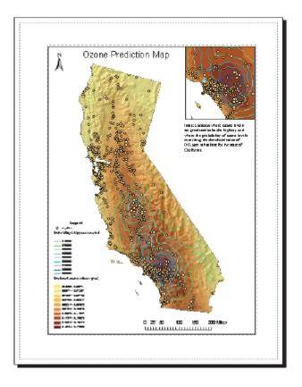
The map shows that the area east of Los Angeles has the highest predicted levels of ozone and the highest probability of exceeding the critical average threshold (0.12 ppm) in at least one eight-hour period during 1996. Since this is the case in the analysis (but remember the original data has been altered), you may wish to focus on these areas and analyze time series measurements of ozone to accurately identify the areas at potential risk.
