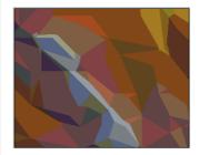
Heterogeneous surfaces that vary sharply in some areas and less in others can be modeled more accurately, in a given volume of data, with a triangulated surface than with a raster. That is because many points can be placed where the surface is highly variable, and fewer points can be placed where the surface is less variable. ArcGIS stores
