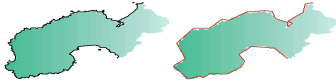
The Generalize method reduced the number of vertices in this shape from 427 to 29.
