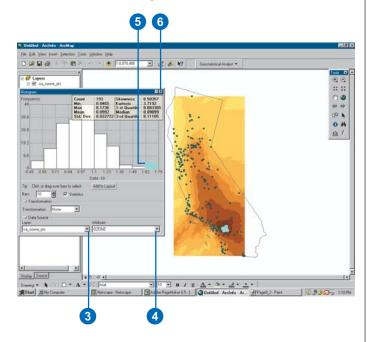
The distribution of the ozone attribute is depicted by a histogram with the range of values separated into 10 classes. The relative proportion (density) of data within each class is represented by the height of each bar.
