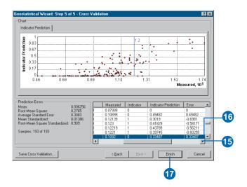
The measured and indicator columns display the actual and transformed values for each sample location. The indicator prediction values can be interpreted as the probability of exeeding the threshold. The indicator prediction values are calculated using the semivariogram modeled from the binary (0,1) data, created as indicator transformations of your original data. Cross-validation sequentially omits a point and then calculates indicator prediction values for each.
