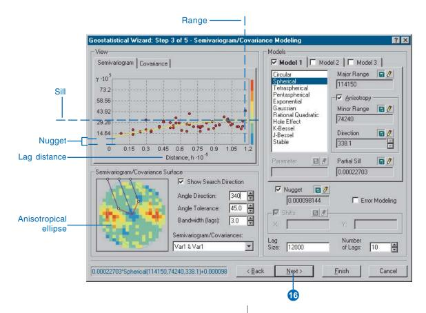
between pairs of points. Points separated by a lag distance greater than the range are spatially uncorrelated. The nugget represents measurement error and/or microscale variation (variation at spatial scales too fine to detect). It is possible to estimate the measurement error if you have multiple observations per location, or you can decompose the nugget into measurement error and microscale variation by checking the Nugget Error Modeling check box.
