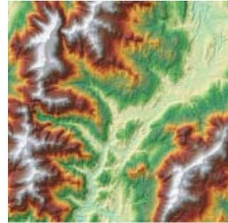
By placing an elevation raster on top of a created hillshade, then making the elevation raster transparent, you can create realistic images of the landscape. Add other layers, such as roads or streams, to further increase the informational content in the display.
