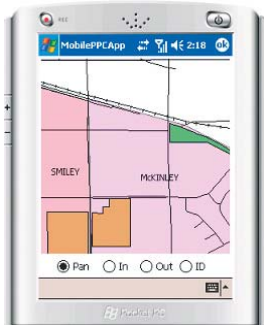
Example of the embeddable mobile map control used for programming mobile map applications with ArcGIS Mobile. The map control displays the mobile map and includes tools for map interaction and use.
