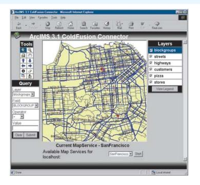
The ColdFusion Template is composed of a series of files that open in sequence. The starting page, index.cfm, initializes the application, then calls ai\_Frameset.cfm, which divides the main page of the template into seven frames—TopFrame, ToolFrame, QueryFrame, MapFrame, ServicesFrame, LayersFrame, and BottomFrame.
