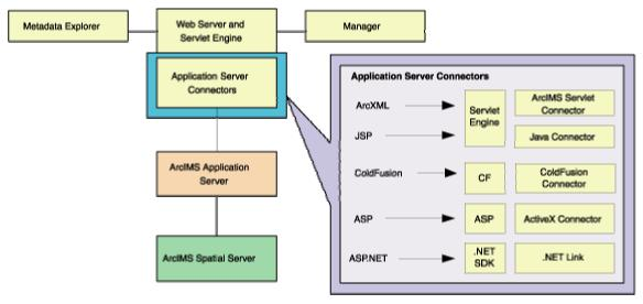
The ArcIMS Servlet Connector is the standard connector used for ArcIMS. It uses the ArcIMS language, ArcXML, to communicate from the Web server to the ArcIMS Application Server. The ArcIMS Servlet Connector provides Map Service-level user password authentication. You need the ArcIMS Servlet Connector to administer your ArcIMS site and author and design ArcIMS Web pages. The WMS connector for ArcIMS enables ArcIMS to work within the OCG WMS specification.
