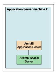
This machine will be identical to Application Server machine 1. If used for round-robin, it will rotate requests among the two Application Servers. If used for failover, it will serve maps when Application Server machine 1 is inaccessible. This machine, like Application Server machine 1, will host ArcIMS Application Server and ArcIMS Spatial Server. Service Administrator will be used to administer the Application Server.
