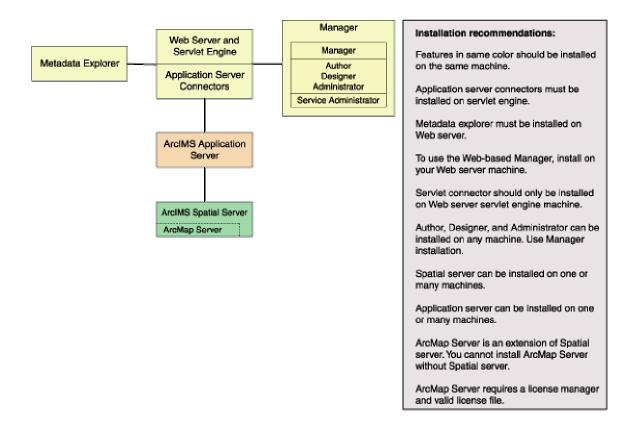
When planning your ArcIMS site configuration, there are some installation recommendations to take into account. The installation configuration diagram above illustrates ArcIMS installation features and some of the installation recommendations.
