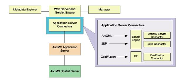
The Servlet Connector is the standard ArcIMS Connector. The typical installation installs this connector. You need this connector if you plan to administer Web pages or use the Web design tools in ArcIMS (Author and Designer). The Servlet Connector also provides MapService-level user password authentication.
