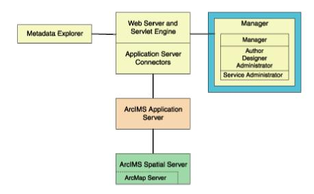
ArcIMS Manager Applications are installed with the typical installation; you only need one ArcIMS Manager installation per site.
