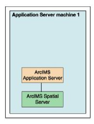
This will be the main Application Server machine. This machine will host the ArcIMS Application Server and the ArcIMS Spatial Server. The service Administrator will be used to administer this ArcIMS Application Server. We will also create an identical set up on another machine, which will be the back-up machine for failover.
