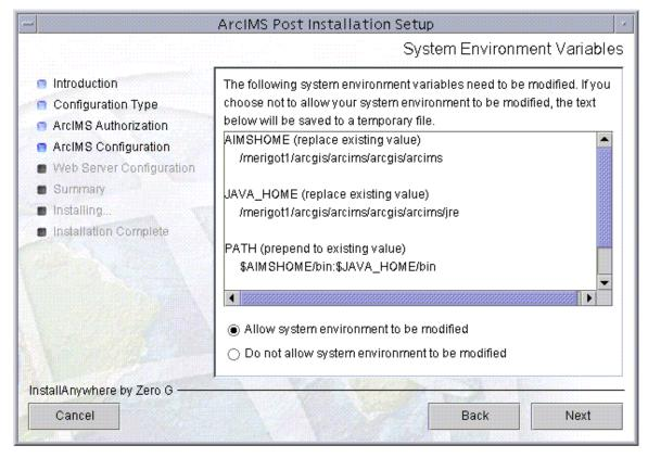
A list of required edits is displayed. The post installation setup can make these changes to your system environment variables for you. If you do not allow the post installation setup to make these edits, to successfully complete your ArcIMS installation you must make the edits manually. A temporary file containing the necessary edits is created for you. The temporary file is located at: \$HOME/ArcIMS\_envVars.txt.
