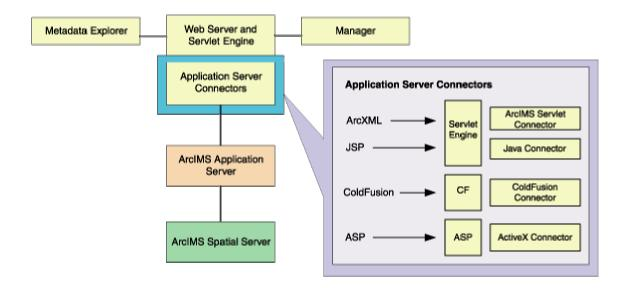
The ArcIMS Servlet Connector is the standard connector used for ArcIMS, and it supports the Open GIS Consortium (OGC) Web Map Service (WMS) 1.1.0 implementation specification. It uses the ArcIMS language, ArcXML, to communicate from the Web server to the ArcIMS Application Server. The ArcIMS Servlet Connector provides Map Service-level user password authentication. You need the ArcIMS Servlet Connector to administer your ArcIMS site and to author and design ArcIMS Web pages.
