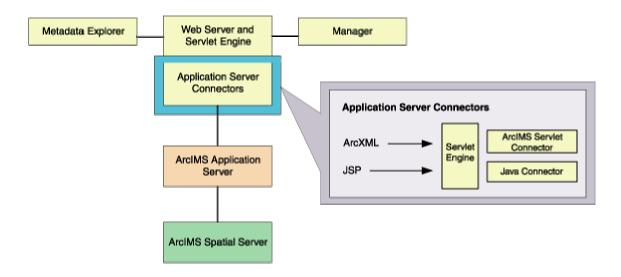
The Servlet Connector with WMS is the standard ArcIMS Connector. Select this connector if you plan to use the Web design tools in ArcIMS (Author and Designer). The Servlet Connector also provides service-level user password authentication. WMS works within the OGC WMS 1.0.0 specification.
