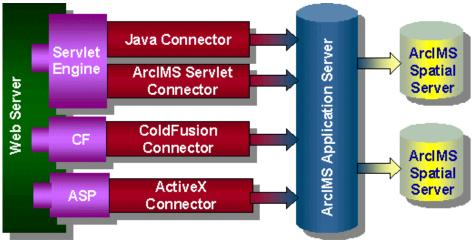
The ArcIMS Servlet Connector is the standard connector used for ArcIMS, and it supports the OpenGIS Consortium (OGC) Web Map Service (WMS) 1.1.0 implementation specification. It uses the ArcIMS language, ArcXML, to communicate from the Web server to the ArcIMS Application Server. The ArcIMS Servlet Connector provides Map Service-level user password authentication. You need the ArcIMS Servlet Connector to administer your ArcIMS site and author and design ArcIMS Web pages.
