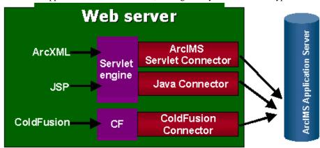
The Servlet Connector with WMS is the standard ArcIMS Connector. Select this connector if you plan to use the Web design tools in ArcIMS (Author and Designer). The Servlet Connector also provides service-level user password authentication. WMS works within the OGC WMS 1.0.0 specification.
