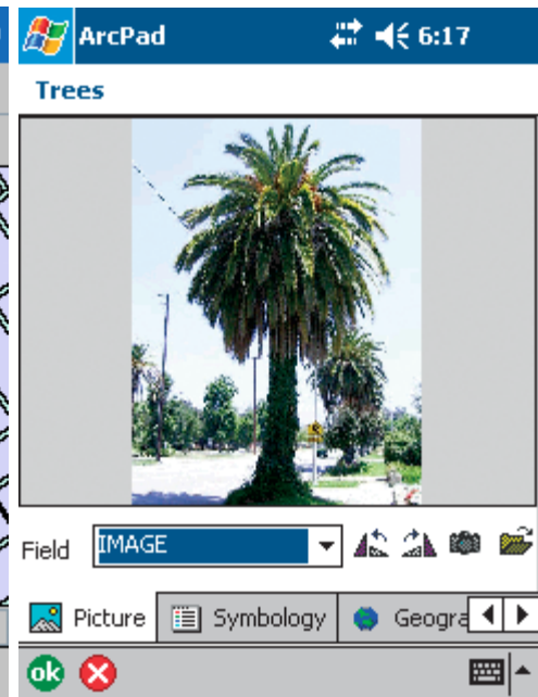
ArcPad enables you to capture photos in the field using a connected digital camera. The photos are then immediately associated with features in a layer.
