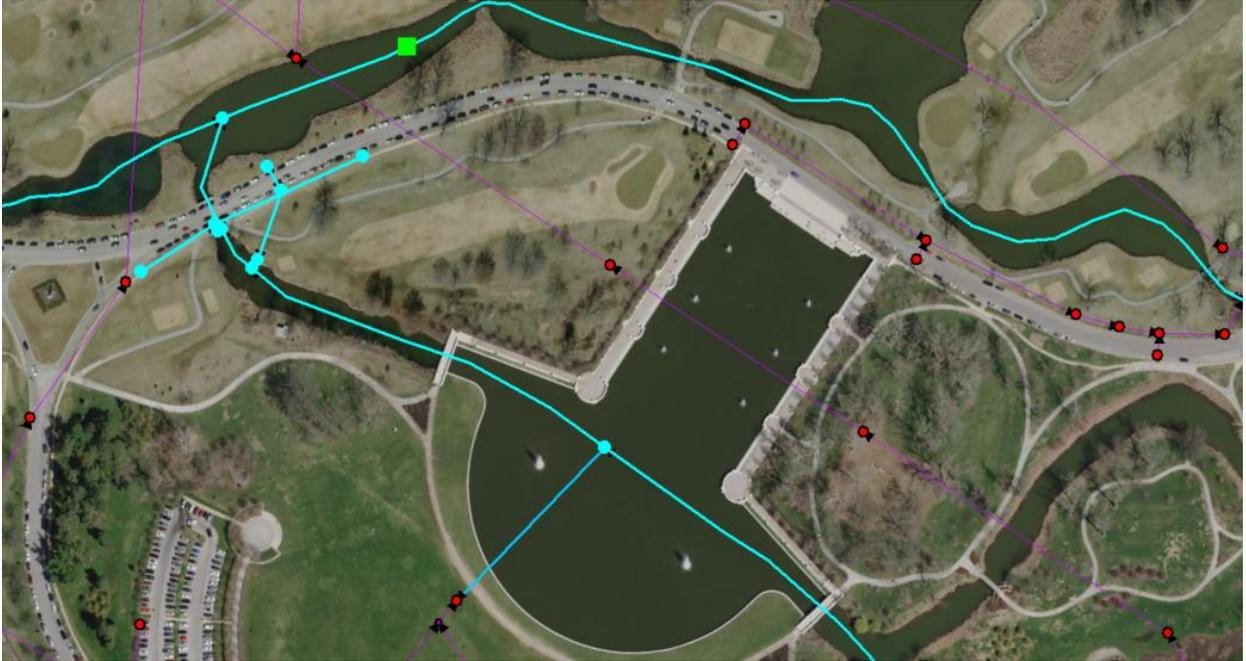
Missing HydroJunction at the end of the blue line.
