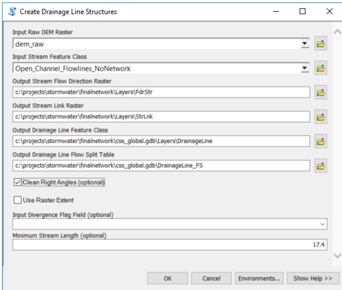
Figure 31 - Create Drainage Line Structures Interface
