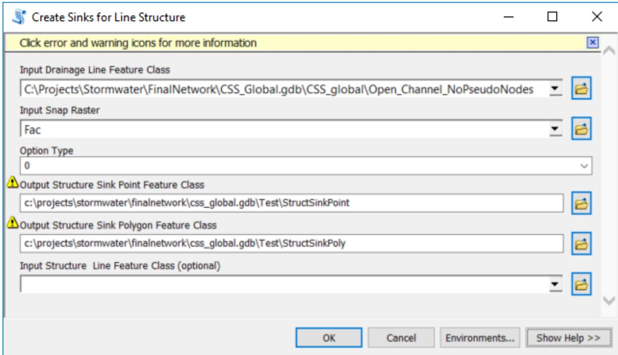
Figure 23 - Create Sinks for Line Structure tool
