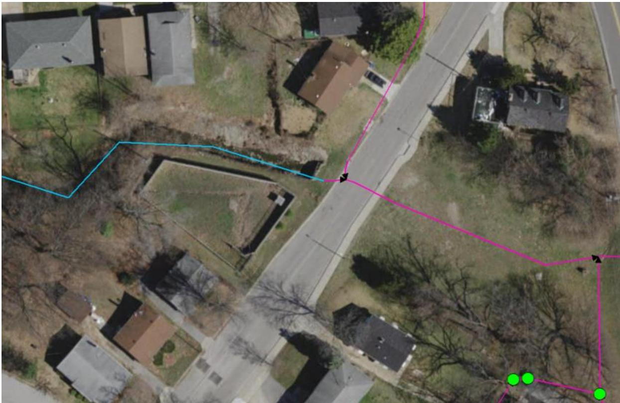
Figure 20 - Missing HydroJunction at end of Terminal Stream
