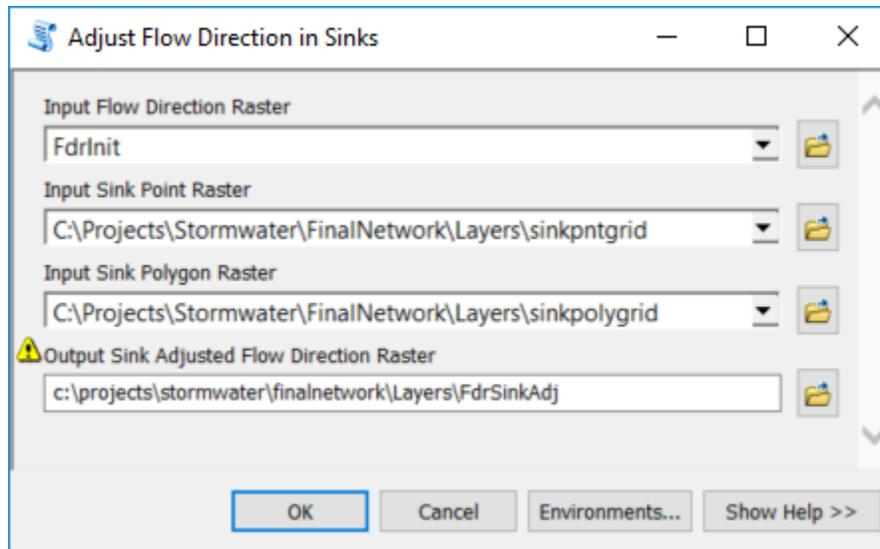
Figure 41 - Adjust Flow Direction in Sinks Interface
