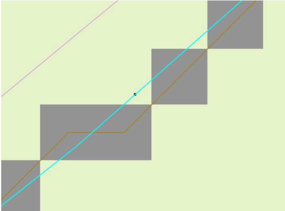
Stream does not match DrainageLine/StrLnk perfectly. But if point is snapped to line for tracing, it should also be snapped to the stream grid for local delineation (snap to closest stream cell).
