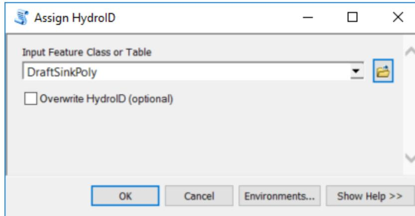
Potential Sinks created. HydroID will be used by the tool Create Sink Structures.
