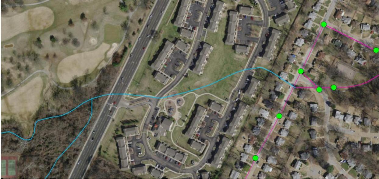
**Figure 21 - Missing HydroJunction at end of Terminal Stream**
