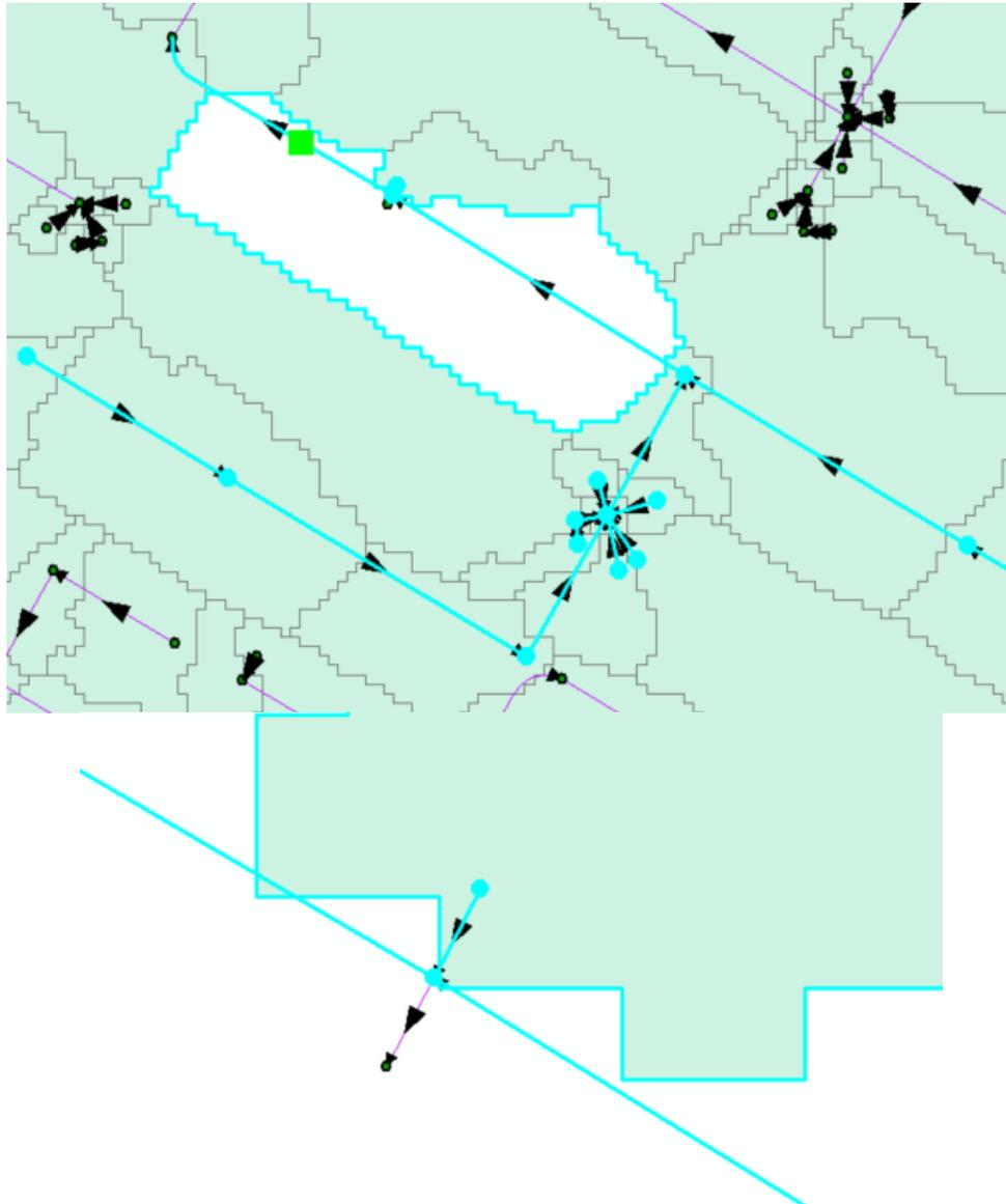
Hole in the watershed cause by wrong flow direction. Need to reverse the direction of the line to fix this issue so the water goes from the lower HydroJunction towards the main pipe instead of away from it.
