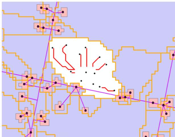
Problem was offset in Level DEM was too small (the z factor was not set properly). To avoid this issue, use a large value for the offset to make sure the elevations in the sink are much lower than any neighboring elevations.
