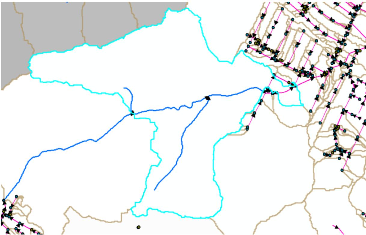
**Figure 22 - Missing Catchments due to filled in stream**
