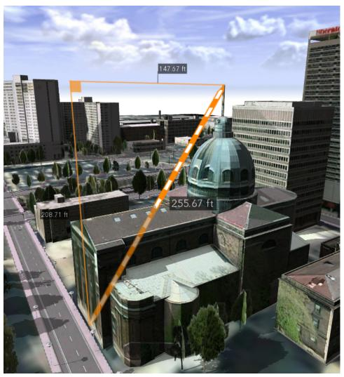
Line of sight, vertical, and horizontal distance are measured. Note: The line of sight shines through the building.
