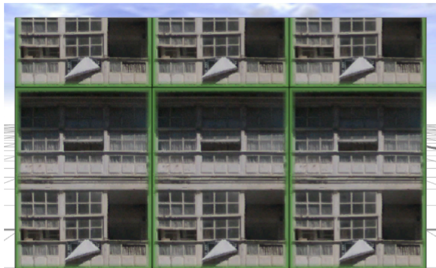
Dimension is shown using Absolute texture width 5.75, Absolute texture height 8.0, Align to Bottom right corner and snap horizontally to bounds, so the texture fits exactly three times.
