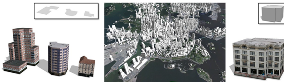
Buildings generated from footprints (first), OpenStreetMap data (middle), and 3D mass models (last) are shown.
