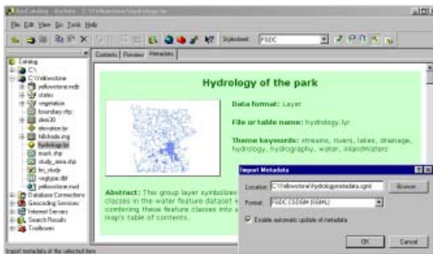
Figure 9. ArcCatalog automates much of the work in documenting data. Simply point ArcCatalog at the data to automatically populate its inherent metadata properties (e.g., coordinate system, feature class, and attribute field names).
