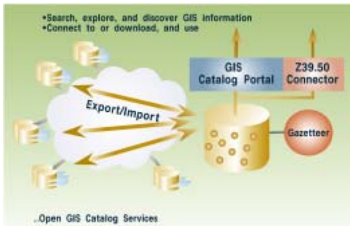
Figure 7. Each GIS catalog portal must support standard searches. Portals often contain support for various search mechanisms, including standard Web portal searches as well as Z39.50.
