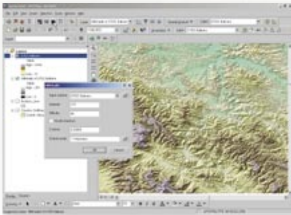
Using the DTED Tool, the applicable DTED tiles can be automatically selected and merged into a single grid. A hillshade may be applied for ease of interpretation and display. The resultant elevation matrices can be used in subsequent analysis applications.
