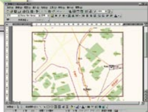
A sample map of the Nanjing City distribution power network shows poles, lines, and transformers.
