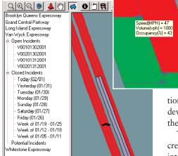
When roadway sensors indicate abnormal traffic flow, the ATMS automatically displays a map to show JTOC operators possible trouble spots (in purple). Operators can zoom in on the map and click icons showing the sensor location to obtain data about traffic speed and volume.
