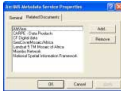
Figure 5 Properties window in ArcCatalog lets you assign related documents to a published data set.
