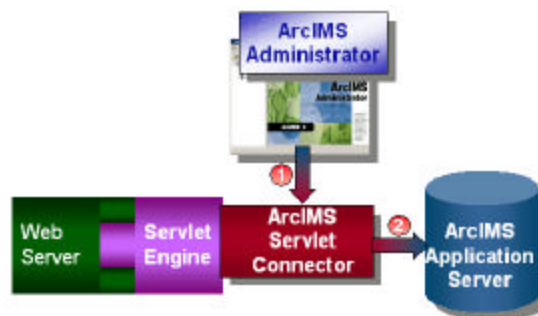
Figure 18 Administrative Requests Are Sent from the Administrator to the ArcIMS Application Server via the ArcIMS Servlet Connector
