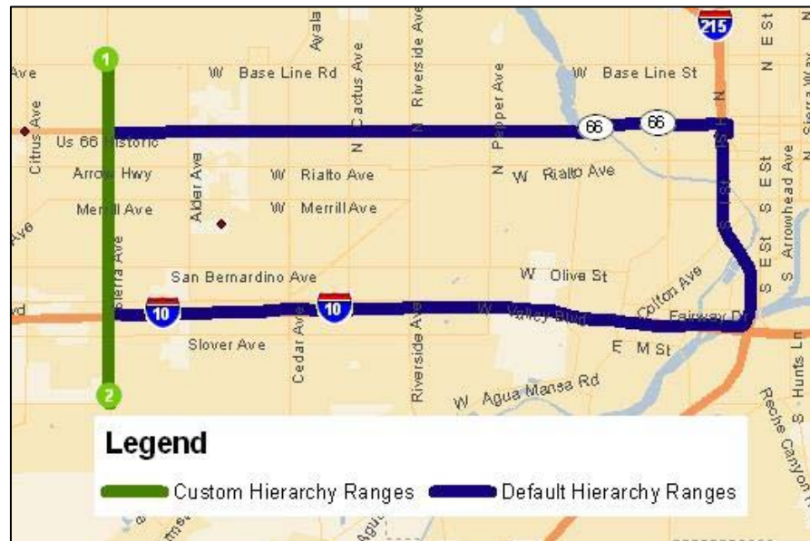
Figure 10 Example of Hierarchical Route Using Default and Custom Hierarchy Ranges
