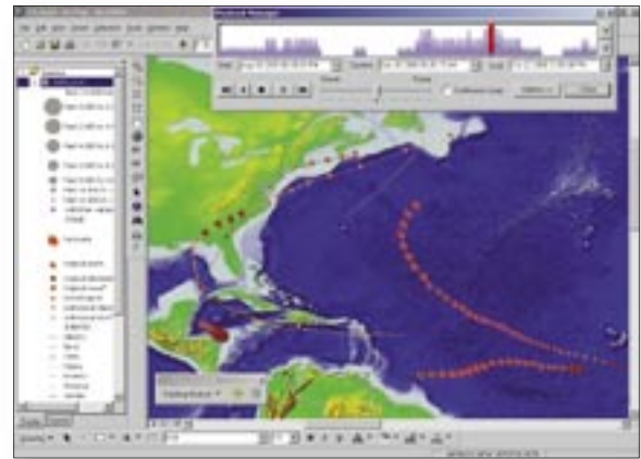
The Playback Manager's Continuous Loop setting recycles the playback to repeat data display. The Animation tool can save playback as an AVI video file or individual frames.
